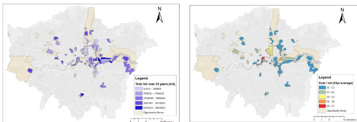
Figure 3: Potential non-potable use (left) and cost per m<sup>3</sup> of non-potable water (right)
